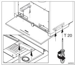
■ Tighten the four securing screws from below.
